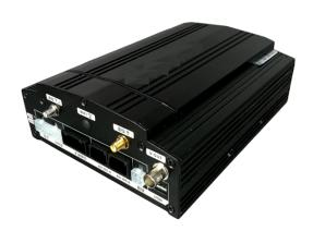
The industrial-quality and fanless design of KVS8713HEB 3.0 enables the easy dissipation of heat. It could endure the voltage surge in vehicle due to the advance power module design and strict quality testing, which is an ideal solution for vehicle surveillance.
